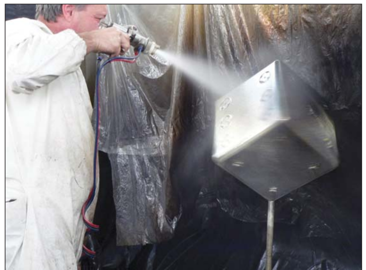
A prop for a window display—made of wood, no less—receives the sprayed-on silvering fluid.
