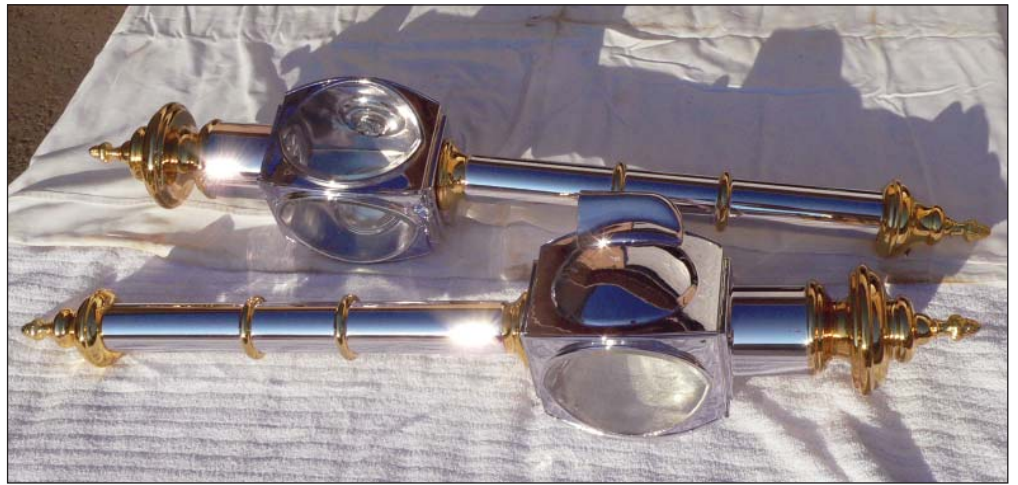
Exterior lamps from a hearse show the bright reflectivity that the new process achieves. The brass-colored highlights were achieved by tinting the clear coat.
